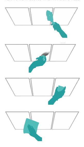
Dust and loose dirt can be easily removed from the face of the ceiling tile by the use of a soft brush or with a vacuum cleaner. A vacuum cleaner fitted with an upholstery attachment is the most suitable. It is recommended that when brushing or vacuuming it is done in one direction only for best results.
